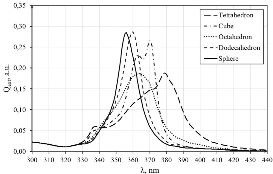
Fig. 5. The effective cross section extinction of the regular polyhedrons and the sphere of the same volume.
