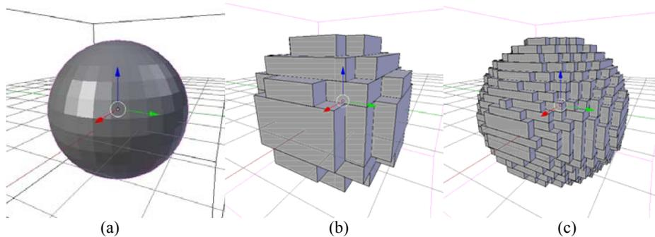
Fig. 1. The voxel mesh generated for 6 nm radius sphere (a) with resolution (b) 0.7 nm per voxel side and (c) 0.3 nm per voxel side.
