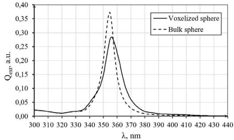
Fig. 2. Comparison of the effective cross section extinction spectra of the voxelized and bulk sphere.
